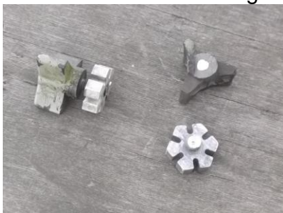
9-8 Club house awning repair - East Brace lock seized, replaced with new (both)
