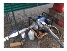
5-7 Fuel tank removed and pump connected to external fuel tank.
