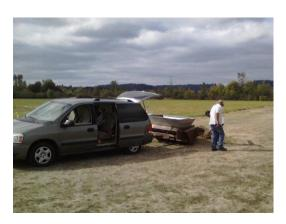
4-29-16 Flat tire pumped up, Warren put a strap around it and then added air, it sealed to the wheel and is holding air.
