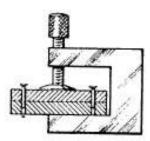
Before laminating plywood for firewalls, lightly clamp and drill two holes a shade smaller than the two nails. Glue the pieces together, tap in the nails to prevent the parts from skidding, then clamp firmly. Once the glue is set, remove the nails and fill the holes. Roy McGuckin, Fairport, New York.
